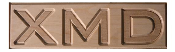
The multi-layer drawings can be prepared in either plt or dxf. When preparing your drawing, color code the different layers. Later on you will set the cutting depth for each color in the MegaCut software.
